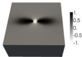
Transmembrane potential at the endocardial surface (top) where anodal stimulus is applied, i.e. inside the white region at the center.
