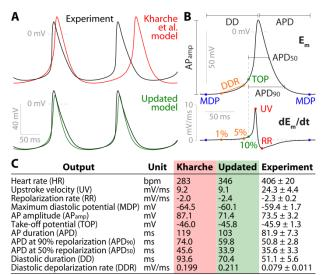
Figure 1. Comparison of experimental and simulated APs. A) Representative APs recorded from a mouse SAN cell (black), and simulated APs generated with the Kharche et al. model (red), or our updated model (green). B) Schematic illustration of AP waveform parameters. C) The updated model improves matches to AP waveform parameters. Experimental data are reported as mean  $\pm$  SE (n=10-14).
